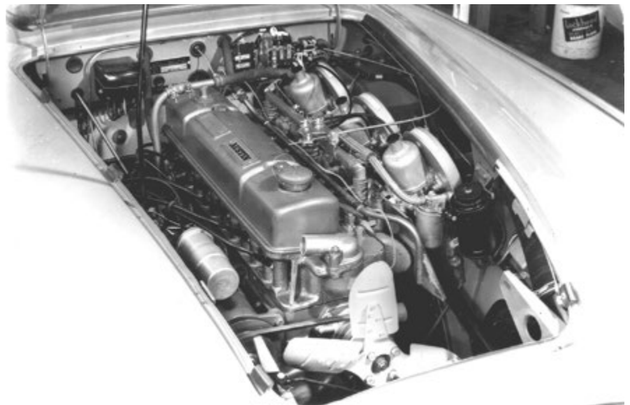
Rare factory publicity photo of tri-carb installation, marked "Confidential until Sept.20." (1960?)
