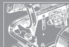
The body number is stamped on a plate secured to the bulkhead between the righthand bonnet hinge and the fuse block.
