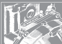
...or it is stamped on a plate secured to the rear of the engine behind the cylinder block. (Twin Cam)
