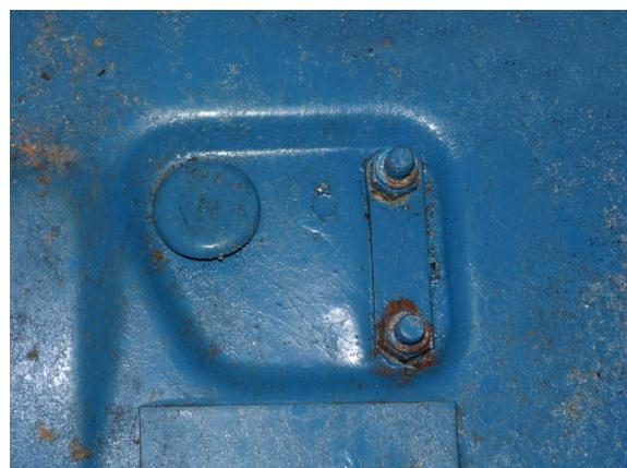
3. Locate the column clamp further up the steering column. This usually has a sheer bolt fitted which must be removed first and a replacement bolt fitted. The easiest way to remove the shear bolt is to slowly tap it with a centre punch in an anticlockwise direction. Please note: The shear bolt shown in the picture has not been 'sheared' for illustration purposes.
