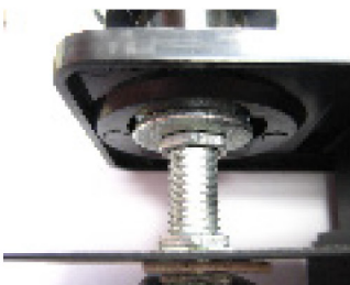
Nuts/Washers Installed Between L Bracket and Faceplate
